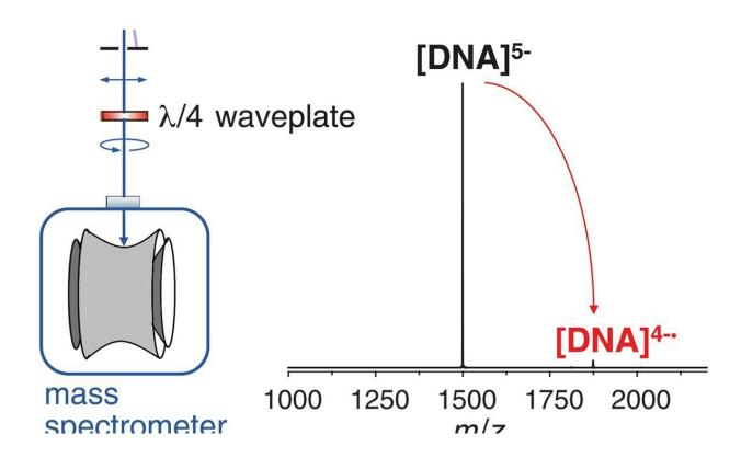
Experimental setup for generating circularly polarized laser pulses. Also shown is the typical mass spectrum after isolation of D-[(dTGGGGT)<sub>4</sub>•(NH<sub>4</sub><sup>+</sup>)<sub>3</sub>]<sup>5-</sup> ions and irradiation with left circularly polarized (LCP) light at 260 nm. See supplementary materials for setup details. Credit: *Science* (2020). DOI: 10.1126/science.abb1822
