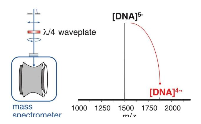
Experimental setup for generating circularly polarized laser pulses. Also shown is the typical mass spectrum after isolation of  $D-[(dTGGGGT)_4 \cdot (NH_4^+)_3]^{5-}$  ions and irradiation with left circularly polarized (LCP) light at 260 nm. See supplementary materials for setup details. Credit: *Science* (2020). DOI: 10.1126/science.abb1822
