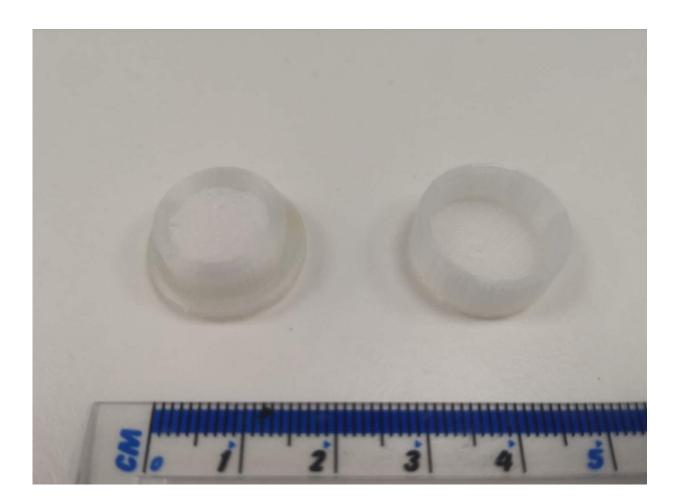
3D printed reservoir used for placing the magnetically actuated sponge and drug to be delivered upon applying a magnetic field. Credit: University of Sussex
