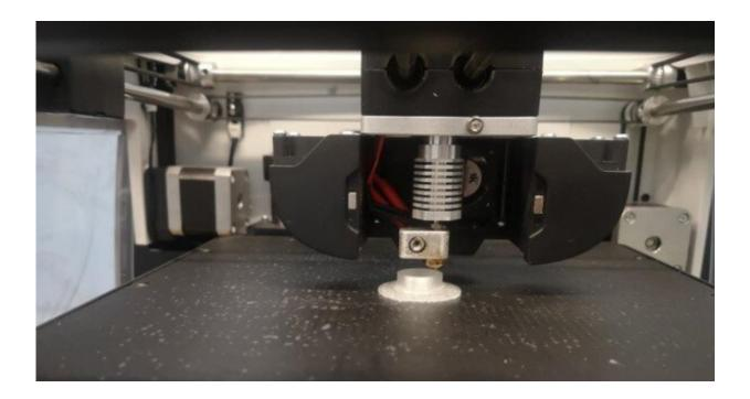
Fabrication of the device reservoir using a standard 3D printing machine. Credit: University of Sussex
