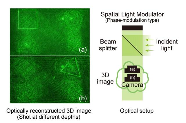
(left) Different images at depths (a) and (b) (see right) show how the distribution of light over space forms a truly 3D image. (right) Schematic of holography setup. The calculated hologram is displayed on a spatial light modulator while laser light is directed to reflect off its surface, interfere with the original beam and form a 3D image at the camera. Credit: Tokyo Metropolitan University
