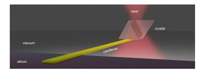
University of Washington researchers used an infrared laser to cool a solid semiconductor material—labeled here as "cantilever"—by at least 20 degrees C, or 36 F, below room temperature. Credit: Anupum Pant
