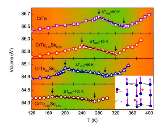
Temperature dependence of volume changes of Cr-Te-Se with different compositions. Credit: ZHENG Xinqi
