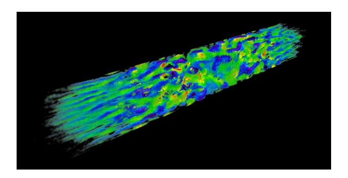
To study the powerful shock waves in supernova remnants, Frederico Fiuza and colleagues created similar plasma shock waves in the lab. Here, computer simulations reveal the turbulent structure of the magnetic field in two shock waves moving away from each other. Credit: Frederico Fiuza/SLAC National Accelerator Laboratory
