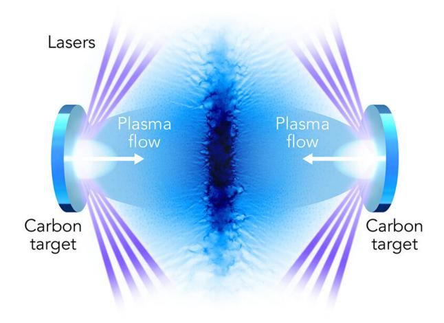
To mimic the shock waves in a supernova remnant, SLAC researchers and their colleagues fired powerful lasers at the National Ignition Facility at two carbon targets, sending two plasma flows into each other. Where they met, the plasmas formed shock waves similar to what's seen in astrophysical shocks. Credit: Greg Stewart/SLAC National Accelerator Laboratory
