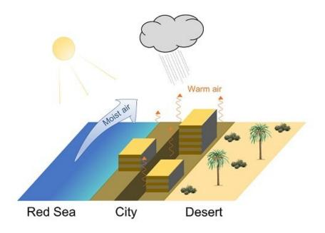
The urban heat island effect causes increasing rainfall over Jeddah. In the city, roads and concrete canyons absorb sunlight; urban surfaces enhance turbulence; warm air rising from the city may collide with moist air from the Red Sea to increase urban rain by 26 percent more than the desert. Credit: 2020 KAUST
