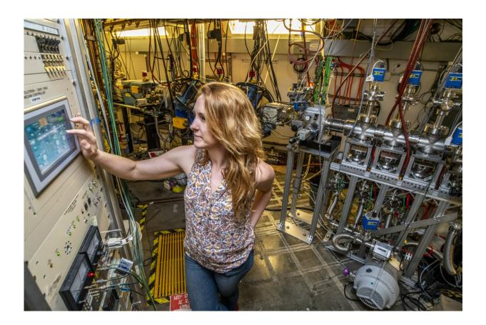
Jennifer Pore, a Berkeley Lab project scientist who led the study detailing the discovery of mendelevium-244, operates the Berkeley Gas-filled Separator vacuum controller at Berkeley Lab's 88-Inch Cyclotron in this 2018 photo. Credit: Marilyn Sargent/Berkeley Lab
