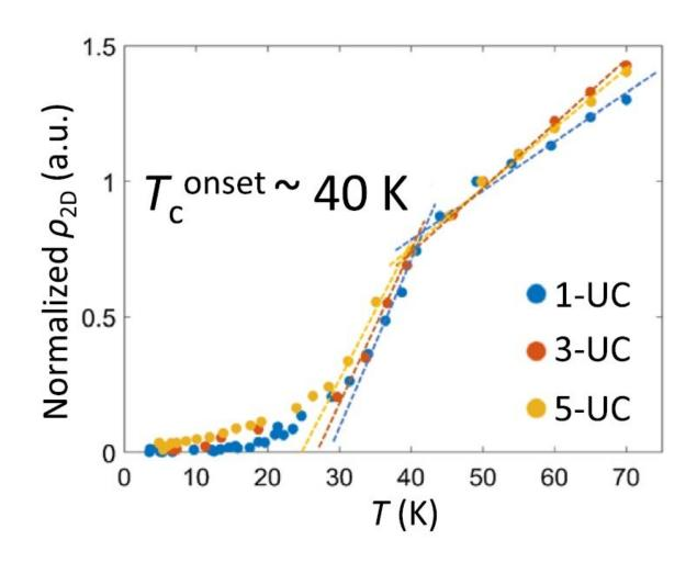
The results show that resistivity begins to decrease sharply at temperatures below 40 K regardless of the thickness of the FeSe layer. This means that twodimensional superconductivity in FeSe/STO occurs at the interface rather than across all FeSe layers.  $\rho$ 2D: two-dimensional resistivity, UC: unit-cell thickness. Credit: Physical Review Letters
