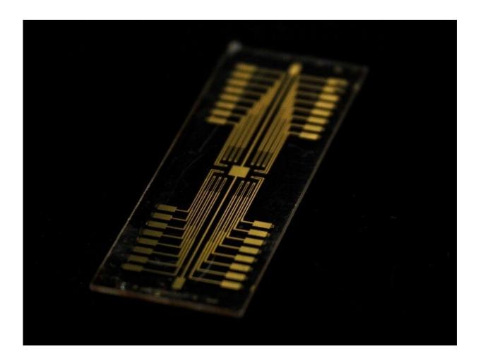
Photograph of a neuromorphic device used in this study. Credit: Shunsuke Yamamoto
