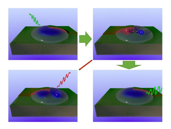
An electron inside a quantum dot is raised by a photon (green waveform) to a higher energy level. The result is a so-called exciton, an excited state consisting of two electrons and one hole. By emitting a photon (green waveform), the system returns to the ground state (green path). In rare cases, a radiative Auger process takes place (red arrow): an electron stays in the excited state, while a photon of lower energy (red waveform) is emitted. Credit: RUB, Arne Ludwig
