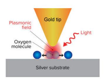
Chemists at RIKEN have discovered how plasmons generated by shining light at the gap between a gold tip and a silver surface and can break the bonds of oxygen molecules adsorbed on the surface. Credit: RIKEN Surface and Interface Science Laboratory
