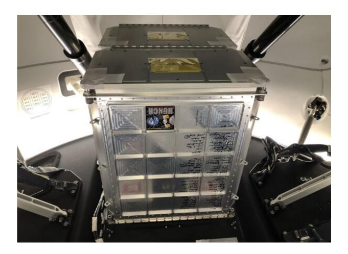
The student-built HUNCH lockers loaded onto the SpaceX Crew Dragon capsule prior to flight. The signatures of students who contributed to the project can be seen on the front of the locker. Credit: SpaceX/NASA
