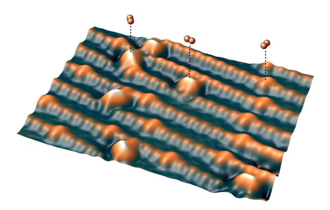
High-resolution picture of the surface: The oxygen adsorbates are clearly visible (orange). Credit: TU Wien
