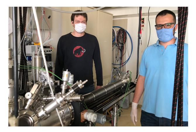
It is extremely difficult to study oxygen molecules on the metal oxide surface without altering them. At TU Wien, this has now been achieved with a special trick: a single oxygen atom is attached to the tip of an atomic force microscope and then it is gently guided across the surface. The force between the surface and the oxygen atom is measured, and an image is taken with extremely high resolution. Credit: TU Wien
