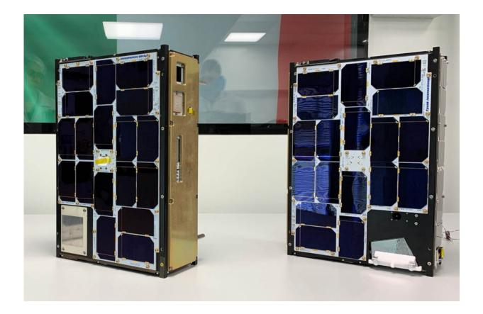
The FSSCat mission is based on two CubeSats, each about the size of a shoebox, that use state-of-the-art dual microwave and multispectral optical sensors to measure, for example, soil moisture, ice extent, ice thickness, urban heat islands and to monitor changes in vegetation and water quality. To take FSSCat to the
