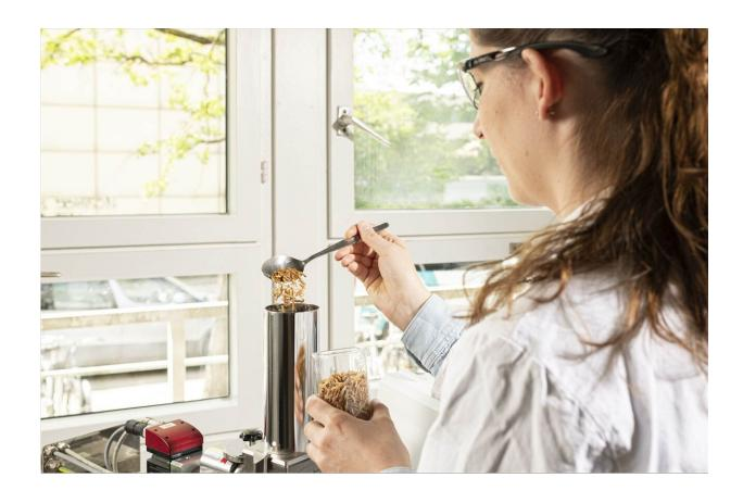
By means of the extrusion method, researchers of KIT study baking properties of insect flours. Credit: Markus Breig, KIT
