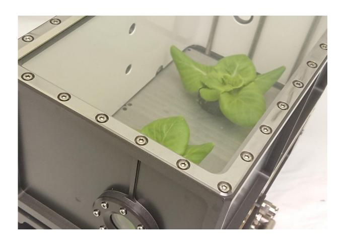
The prototype space greenhouse developed by the TIME SCALE project, which recycles nutrients to grow food. Credit: Karoliussen/HORIZON
