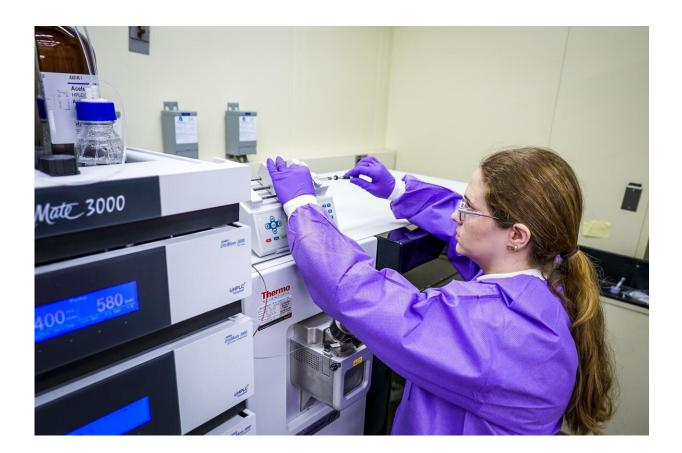
NIST research chemist Kelly Telu injects a sample into a mass spectrometer, a laboratory instrument that scientists use to identify unknown chemical compounds. Credit: M. Delorme/NIST
