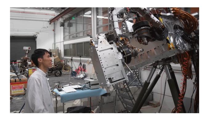
JPL engineers monitor testing of the Perseverance rover's Sample Caching System in this video clip. For the full video, see below. Credit: NASA/JPL-Caltech
