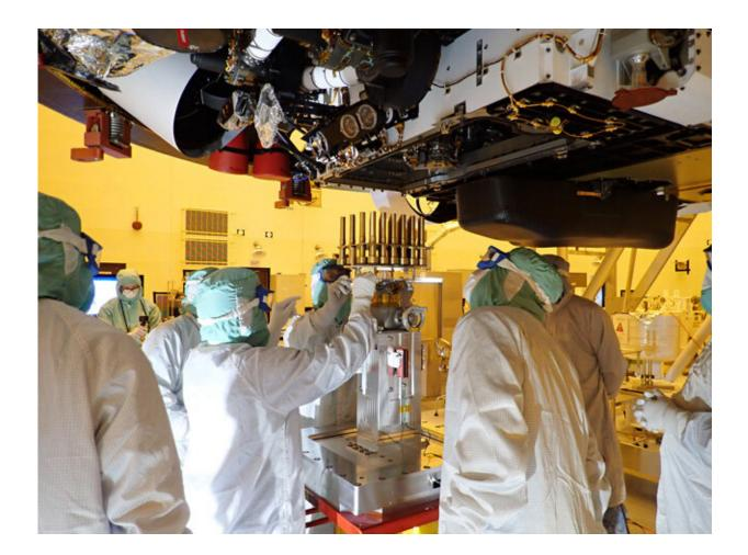
Engineers and technicians working on the Mars 2020 Perseverance team insert 39 sample tubes into the belly of the rover. Each tube is sheathed in a gold-colored cylindrical enclosure to protect it from contamination. Perseverance rover will carry 43 sample tubes to Mars' Jezero Crater. The image was taken at
