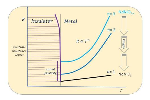
Materials close to a metal-insulator transition (MIT) have great potential in synaptic devices. The figure shows the behaviour of the resistivity of NdNiO<sub>3</sub> as a function of temperature upon changing its oxygen content: the exponent that describes the metallic state can be gradually tuned from n=1 Credit: Beatriz Noheda, University of Groningen
