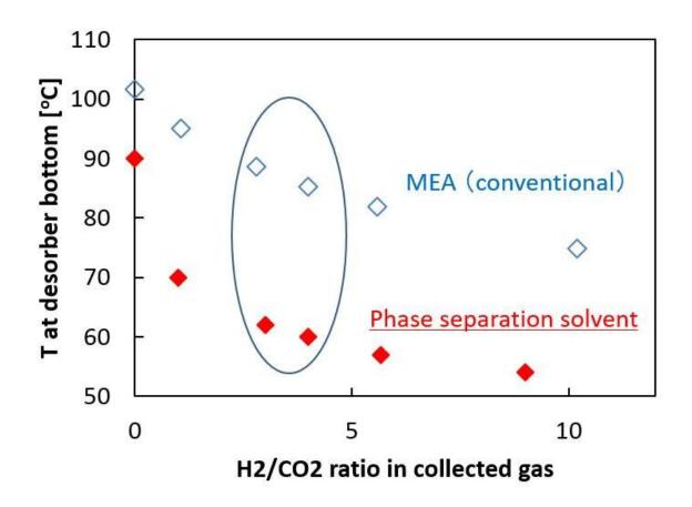
Fig 2. Comparison of H2/CO2 ratio in collected gas and temperature reduction in desorber As the H2/CO2 ratio increases, the temperature at the bottom of desorber will decrease. Stoichiometrically, the ideal H2/CO2 ratio is 4 for the
