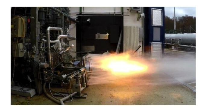
A gas generator produced by additive layer manufacturing completed two test campaigns in 2017 and 2018 at the P8 test bench at the DLR German Aerospace Center's Lampoldshausen testing facility which provided valuable information on the proposed innovative design. Credit: ArianeGroup
