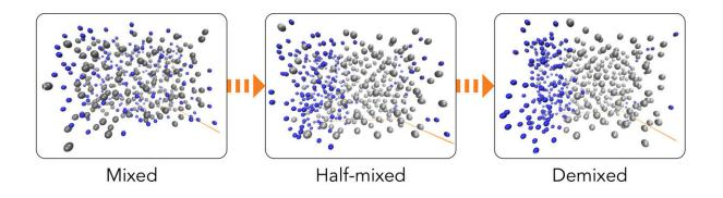
The two sets of scattered photons revealed how hydrogen (blue) and carbon (grey) atoms separated, or demixed, in response to the extreme pressure and temperature conditions reached in the experiment. Credit: Greg Stewart/SLAC National Accelerator Laboratory
