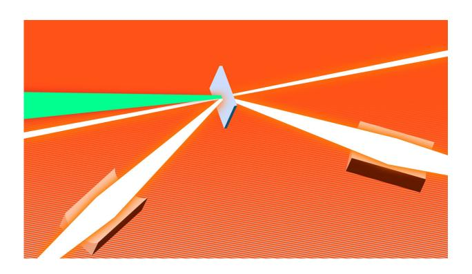
In a new experiment, four optical laser beams (green) launched a shock wave in a plastic sample made up of carbon and hydrogen. As the shock wave moved through the material, researchers observed it by hitting the shocked regions with X-ray photons from LCLS (thin white beam) that scattered both backwards and forwards off electrons in the sample (thicker white beams). Credit: Greg Stewart/SLAC National Accelerator Laboratory
