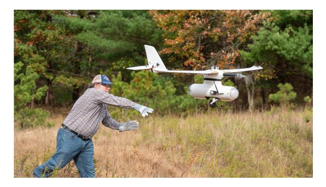
Researchers at Brookhaven Lab are experimenting with an entirely new telescope calibration technique that uses a small, fixed-wing plane. Compared to drones, the plane is faster, can fly for longer periods of time, and can easily fly back to the same point, making it far simpler for researchers to cross-check their results. Credit: Brookhaven National Laboratory
