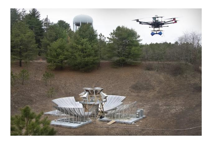
To calibrate the BMX radio telescope, researchers mounted a small radio source to a quadcopter drone and then flew it over the telescope, making a zig-zag pattern over the telescope's entire field of view. By comparing the drone's known flight path from GPS signals to the radio signals picked up by BMX, the researchers are able to determine what signals were missed by the telescope. Credit: Brookhaven National Laboratory
