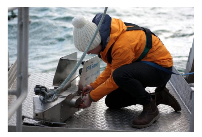
The Continuous Plankton Recorder device is towed in surface waters and occupies a similar space to a marine mammal Credit: Marine Biological Association
