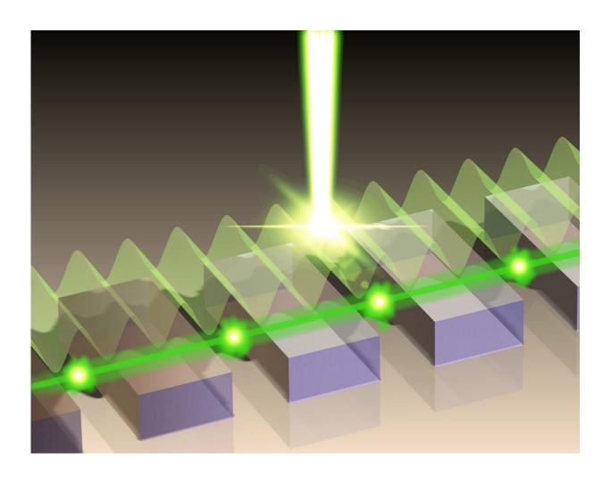
A phase-locking scheme for plasmonic lasers is developed in which traveling surface-waves longitudinally couple several metallic microcavities in a surface-emitting laser array. Multi-watt emission is demonstrated for single-mode terahertz lasers in which more photons are radiated from the laser array than those absorbed within the array as optical losses. Credit: Yuan Jin, Lehigh
