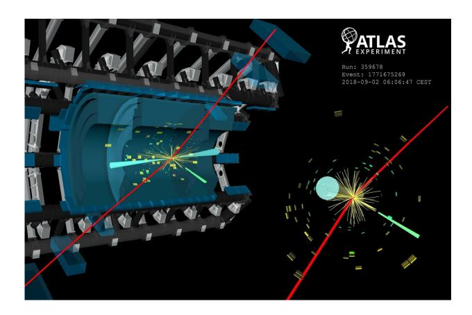
Figure 1: Event display of a candidate Higgs-boson decay to a photon and a Z boson, where the Z boson decays to two muons (shown in red). Green rectangles correspond to energy deposits in cells of the electromagnetic calorimeter, while yellow rectangles correspond to energy deposits in cells of the hadron calorimeter. Credit: ATLAS Collaboration/CERN
