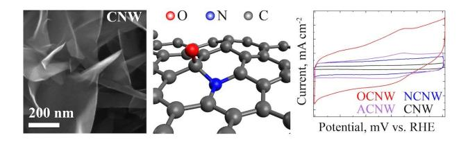
SEM image of Carbon NanoWalls (CNW), a possible position of oxygen and nitrogen heteroatoms, cyclic voltammetry curves in acidic electrolyte. Credit: Skolkovo Institute of Science and Technology
