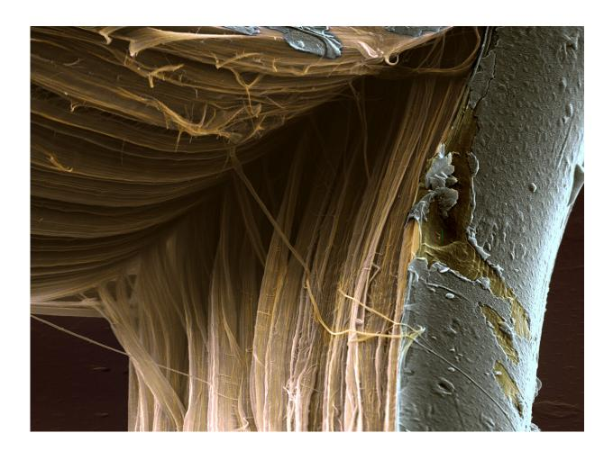
The interior of a high-performance ballistic fiber, illustrating the complex hierarchy within. The split fiber exhibits bridging features, ranging in size from the nanoscale to the microscale, that are offering new insights into fiber failure and could inform the development of next-generation super-fibers. Credit: Joel Brehm / Taylor Stockdale / Yuris Dzenis
