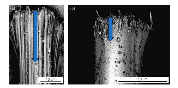
Microscopic views of a polyethylene fiber (left) and a stiffer Kevlar fiber (right) after being stressed. The blue arrowed lines indicate the length of fibrillation in each, showing that bundle separation extended much farther along the length of the former than the latter. Credit: American Chemical Society / ACS Applied Materials and Interfaces
