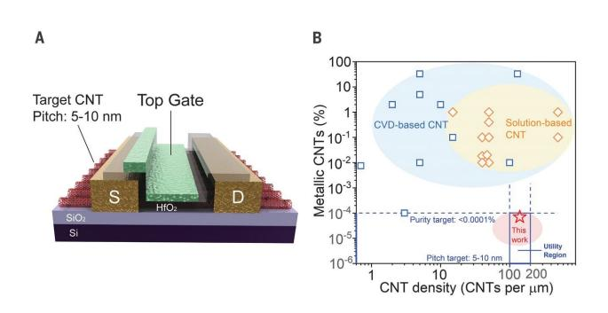
Transistor structure and material target for CNT FET–based digital IC technology. (A) Schematic diagram showing a CNT-based top-gate FET with an ideal 5- to 10-nm CNT pitch. S, source; D, drain. (B) Semiconducting purity versus density of CNT arrays. The utility region is marked as a blue hollow box, and our results are located in the pink region, with a typical one marked as a red star. Credit: *Science* (2020). DOI: 10.1126/science.aba5980
