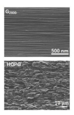
Figure 1. Cross-section scanning electron micrography images of specimen G2800 (top) and a highly oriented pyrolytic graphite (HOPG) specimen (bottom). (Kaneka Corporation, Physical Review Materials (2020))
