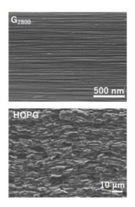
Figure 1. Cross-section scanning electron micrography images of specimen G2800 (top) and a highly oriented pyrolytic graphite (HOPG) specimen (bottom). (Kaneka Corporation, Physical Review Materials (2020))
