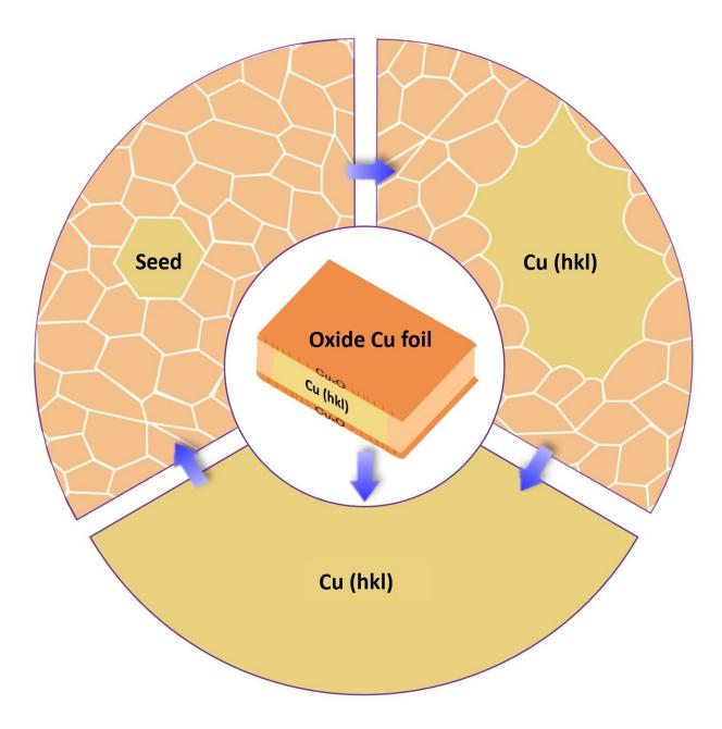
Illustration of the process of obtaining single crystalline Cu foils with different surface structures. Credit: IBS
