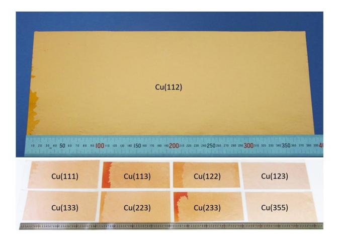
Large area single crystalline Cu foils with high-index surfaces. Credit: IBS
