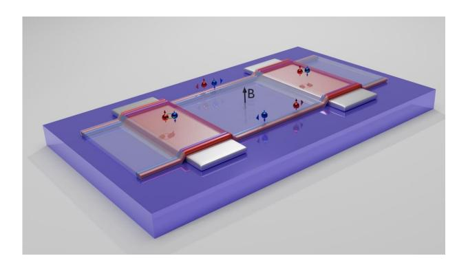
An atomically thin layer of tungsten ditelluride is located between two contacts (in silver). Current only flows through the material in very narrow channels at the outer edges. Credit: Department of Physics, University of Basel
