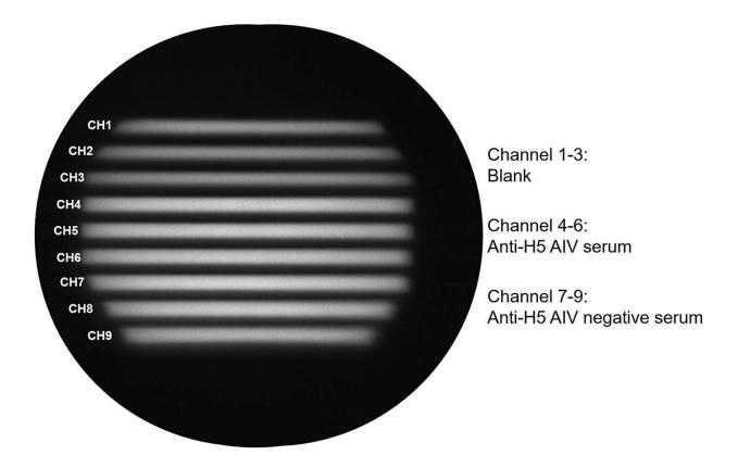
An image obtained by the device and to be analyzed by the image analyzer. Samples show different degrees of polarization of light depending on the presence, absence, or the amount of anti-H5 avian influenza virus antibodies. Credit: Nishiyama K. et al., Sensors and Actuators B: Chemical. April 21, 2020
