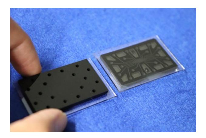
The microfluidic device to which ~20  $\mu L$  of samples containing 2  $\mu L$  of serum will be applied. Credit: Nishiyama K. et al., Sensors and Actuators B: Chemical. April 21, 2020
