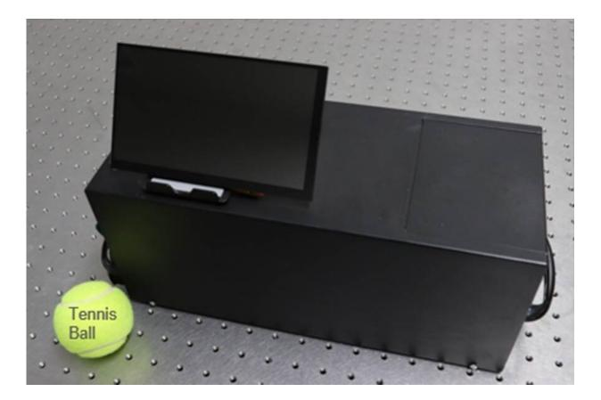
The newly developed portable fluorescence polarization analyzer (35 cm wide, 15 cm high, 15 cm long, and weighs 5.5 kg) combines a microfluidic device, an optical system, a liquid crystal, and an image sensor, enabling the rapid analysis of multiple samples. Credit: Nishiyama K. et al., Sensors and Actuators B: Chemical. April 21, 2020
