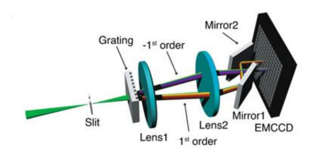
Schematic of the 3D biplane SDsSMLM system. Credit: Northwestern University
