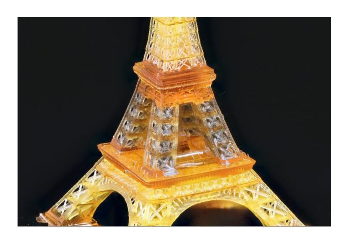
An Eiffel Tower-like 3D structure printed using the researcher's method. Credit: Hensleigh et al
