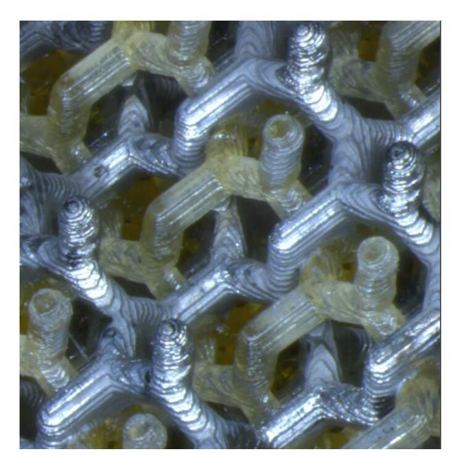
A 3D gyroid-based 3D structure printed using the researchers' method. Credit: Hensleigh et al.
