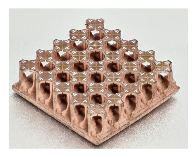
An antenna printed using the researchers' method. Credit: Hensleigh et al.
