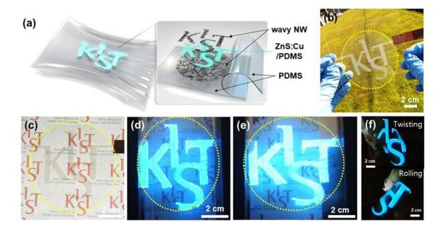
(a-c) Schematic image and photographic images of a logo-patterned stretchable and transparent ZnS:Cu alternating-current electroluminescent (ACEL) device with our wavy Ag nanowire-based stretchable and transparent electrodes. (d-f) Electroluminescent image of stretchable and transparent ZnS:Cu ACEL devices under diverse mechanical deformations, including (e) 40% stretching and (f) twisting and rolling. \* polydimethylsiloxane(PDMS) Credit: Korea Institute of Science and Technology (KIST)
