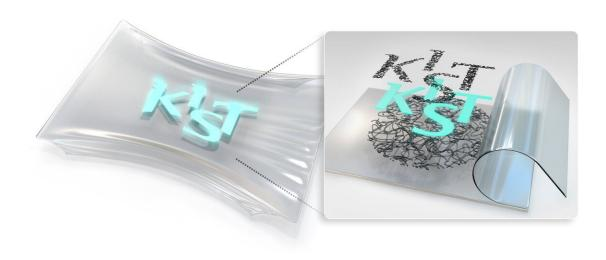
A Korean research team has developed a large-scale stretchable and transparent electrode for the stretchable display. The Korea Institute of Science and Technology (KIST) announced that a research team has developed a technology to fabricate a large-area wavy silver nanowire network electrode that is structurally stretchable with a high degree of conductivity and transparency. Credit: Korea Institute of Science and Technology (KIST)
