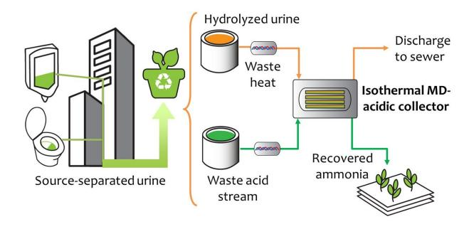
Urine, which contains most the nitrogen excreted by humans, can be isolated at the source via dry urinals and urine-diversion toilets. Through isothermal MD, volatile ammonia in hydrolyzed urine is driven across a hydrophobic microporous membrane where it is recovered as an ammonia fertilizer product in the acidic collector stream. The remaining urine can then be discharged to the sewer. Credit: Ngai Yin Yip and Chanhee Boo/Columbia Engineering
