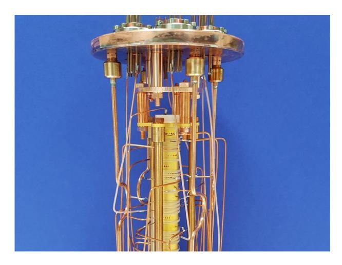
An extremely precise atomic balance: Pentatrap consists of five Penning traps arranged one above the other (yellow tower in the middle). In these identically constructed traps, ions in the excited quantum state and in the ground state can be measured in comparison. In order to minimize uncertainties, the ions are also moved back and forth between different traps for comparative measurements. Credit: MPI for Nuclear Physics
