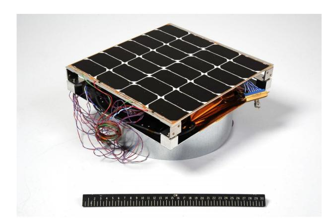
The Photovoltaic Radio-frequency Antenna Module (PRAM) with a 12-inch ruler for scale. The hardware is the first orbital experiment designed to convert sunlight for microwave power transmission for solar power satellites. Credit: U.S. Naval Research Laboratory
