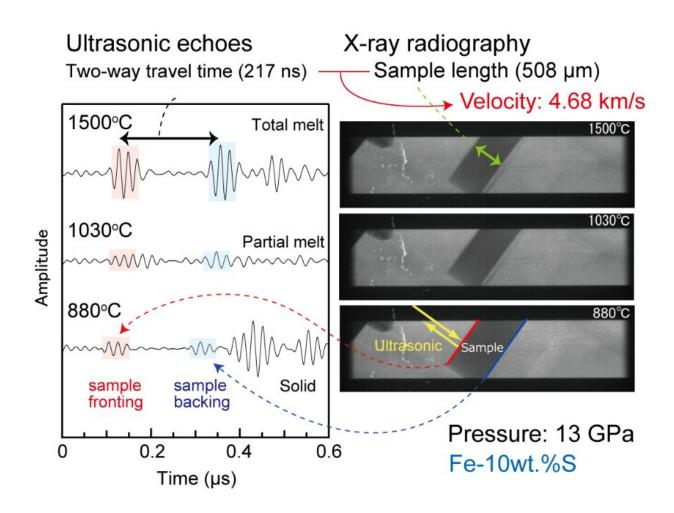
Pulsed waves propagate through samples at the speed of sound. Credit:  $\bigcirc$  2020 Nishida et al.
