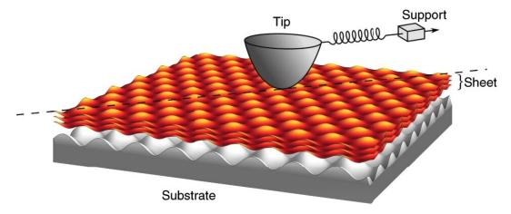
A tip is dragged via a spring over a sheet comprised of a number of atomically thin layers that lie on a substrate but do not slide on it.
