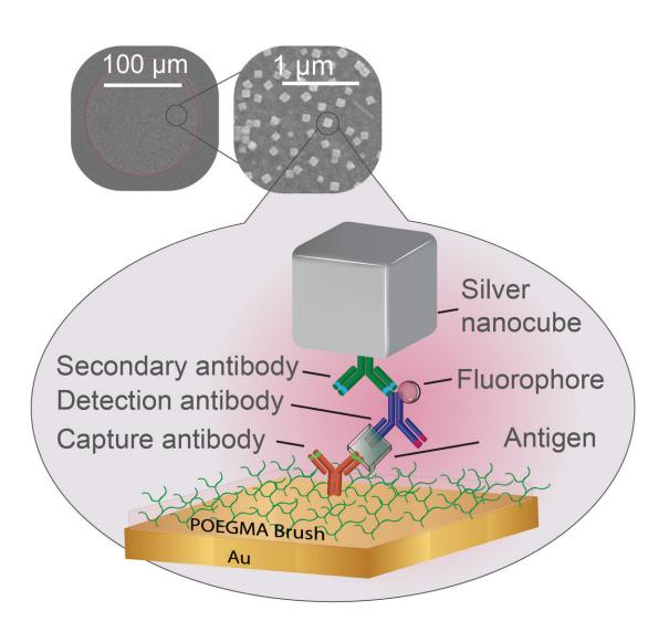
Researchers have shown that plasmonics can enhance the fluorescent markers used to signal positive samples in certain types of tests for diseases. A polymer brush coating keeps unwanted biomolecules away while a capture antibody (red)
