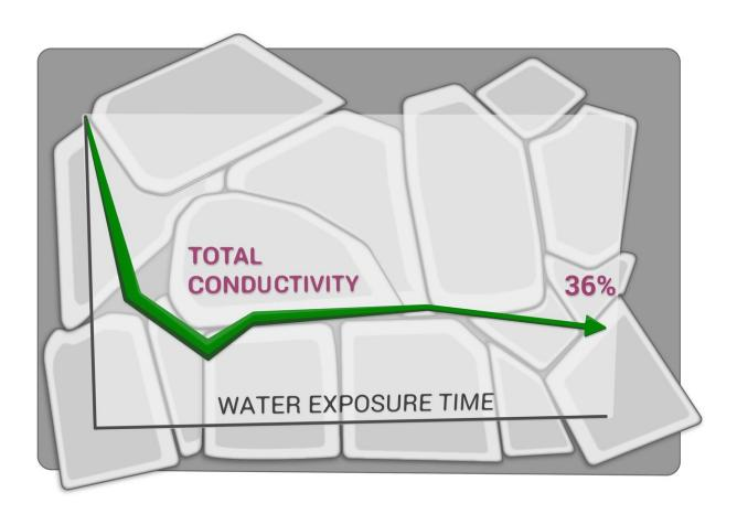
Skoltech researchers and their colleagues have shown that LATP, a solid electrolytes considered for use in next-generation energy storage, is highly sensitive to water, which has direct implications for potential battery performance and lifetime. The paper was published in the journal Chemistry of Materials. Credit: Pavel Odinev / Skoltech
