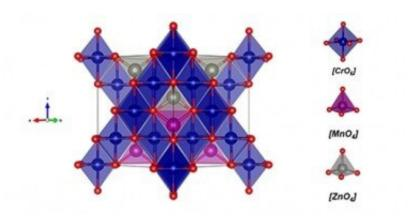
Structure of Mn0.5Zn0.5Cr2O4 molecule with corresponding atom clusters. Thanks to its magnetic properties, the material can be used in a range of products, from gas sensors to data storage devices. Credit: Renan Ribeiro
