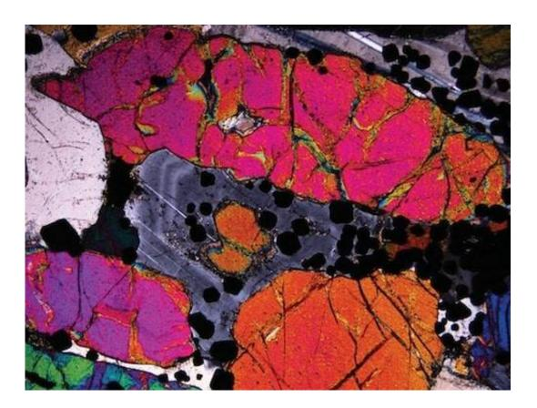
Photomicrograph in crossed polars of precious-metal bearing peridotite. Note the optical zoning (light/dark bands) in the plagioclase (grey coloured mineral) in the central part of the image. The occurrence of this zoning was the focus of the study in question. The width of the image frame is 4 mm. Credit: Nat. Geosci. (2020). https://doi.org/10.1038/s41561-020-0568-3
