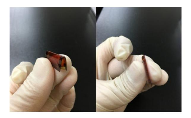
Repeated bending causes irreparable damage to flexible conductors in the form of microscopic cracks. Developing cost-effective ways of addressing this issue is a prerequisite before flexible electronic devices find their way into our lives. Credit: DGIST
