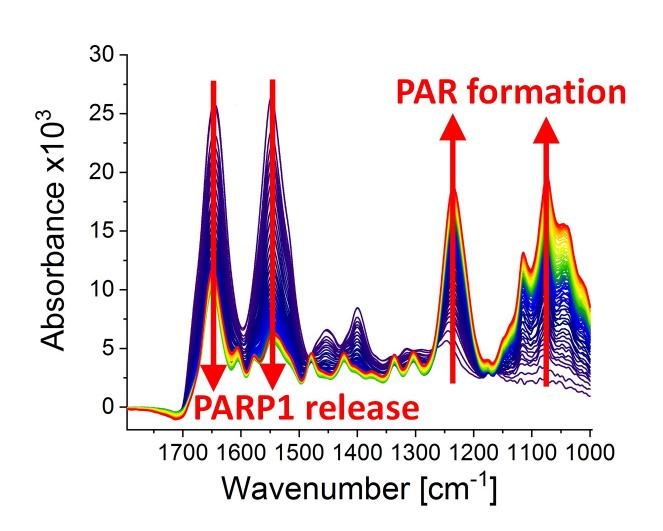
Infrared spectra at different points of time (0-79 min) after the poly(ADP-ribosyl)ation reaction started due to the addition of PARP1 substrate NAD+. The following can be observed: the dynamic formation of the biopolymer poly(ADP-ribose) (absorption bands at 1236 cm-1 and 1074 cm-1) and the detachment of PARP1 from the DNA strand break (absorption bands at 1645 cm-1 and 1548
