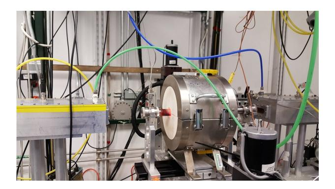
Experimental setup at the Advanced Photon Source, Materials Research Collaborative Access Team's beamline 10-ID for X-ray absorption analysis of electrocatalyst precursors during pyrolysis. Credit: Argonne National Laboratory
