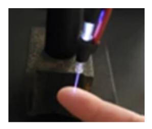
An atmospheric-pressure plasma jet is used for sterilization of antibiotic-resistant bacteria. The plasma is non-thermal and can be applied to living tissue without thermal damage. Credit: Sean Knecht
